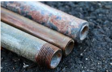
(L-R) Galvanized, Copper, Lead Pipe
