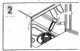
Open door, and remove standpipe from tank.
