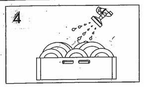
Prescrap wears and load into rack. Do not overload rack.
