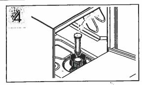
Perform regular cleaning and replace standpipe when finished.
