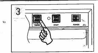
Press and hold "DRAIN" button — until machine has drained.
